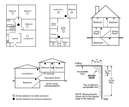
Smoke detectors should always be installed in accordance with NFPA 72, the National Fire Alarm Code. Smoke detectors should always be located in accordance with:
